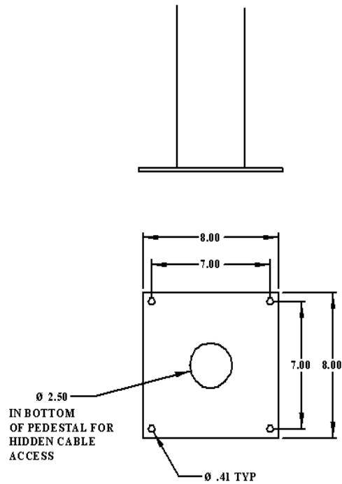
1. Prepare the mounting surface for installation of the pedestal by referring to the illustration above.
