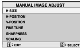
The **Manual Image Adjust** controls are explained below:
