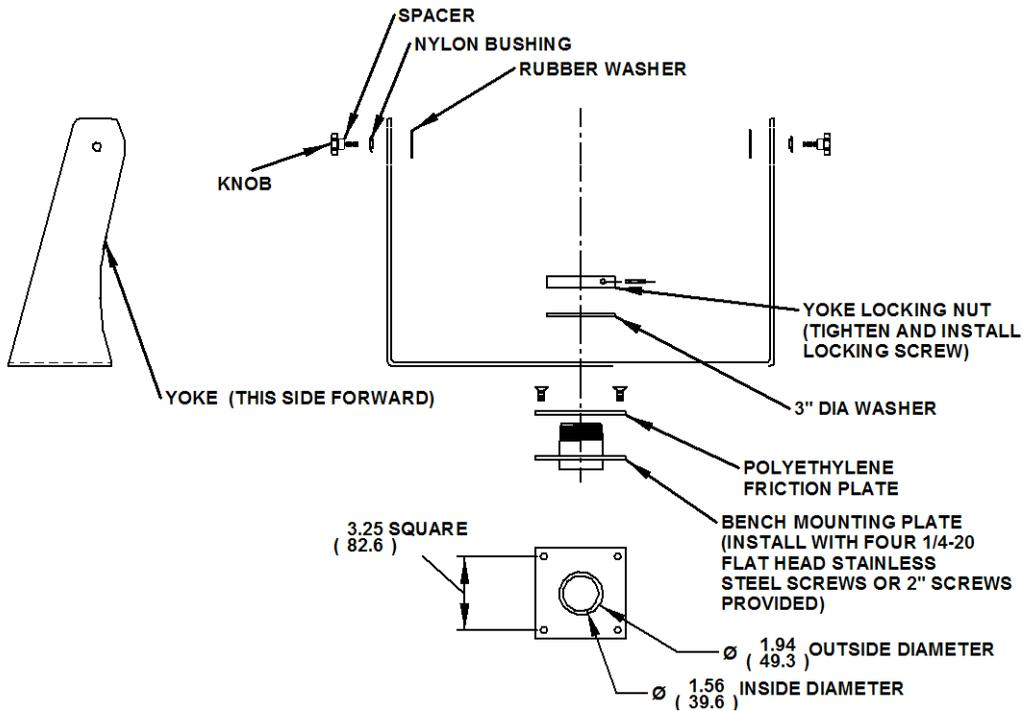
1. Prepare the mounting surface for installation of the bench mounting plate referring to the illustration above.
