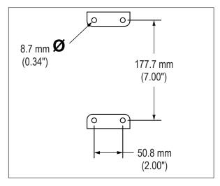
FIGURE 2 – YA \_ \_ -24- \_ \_ MOUNTING PATTERN
