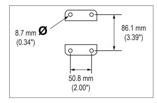
FIGURE 1 – YA \_ \_ -15- \_ \_ MOUNTING PATTERN
