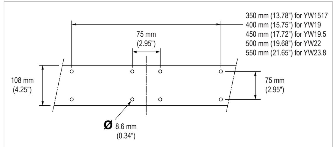
FIGURE 1 – YW \_\_ -07- \_\_ MOUNTING PATTERN
